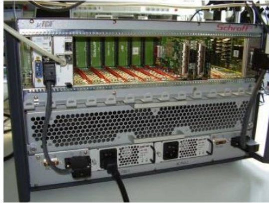
FIGURE 3.4 – Picture of a micro-TCA crate containing DAQ boards with 32 ADC channels/board as developed in 2010.
