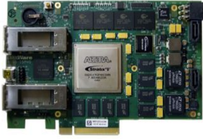
FIGURE 3.6 – FPGA processing board based on Stratix V from Altera. The board features a dual QFP+ cages for 40GigE or 10GigE links, 16 GBytes DDR3 SDRAM, 72 MBytes QDRII/II+, two SATA connectors and is programmable via OpenCL.
