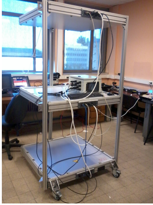
Figure 8. Picture of the muon telescope used for the SHADOW experiment, here during the open-sky calibration phase. The three detection matrices are horizontal. The calibration gives access to the effective acceptance and allows to measure the timing parameters for the time-of-flight measurements. The control box embedding a mini-PC, a common clock distribution system, a network switch is visible on the middle matrix.
