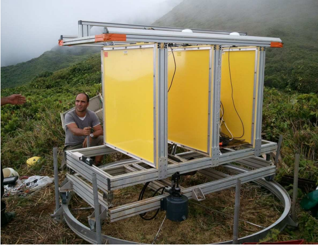
Figure 1. Left : Picture of a muon telescope in horizontal position. The three detection planes are protected by the yellow frames. Right : The inner part of a matrix : active XY scintillator planes, PMT and readout electronics.
