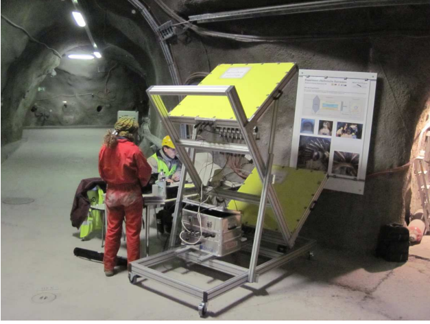
Figure 5. Small-size telescope in operation in the Mont Terri underground laboratory. This telescope is equipped with two 16 \times 16 matrices with 5^2 \text{ cm}^2 pixels separated by D = 120 \text{ cm} for this setup.
