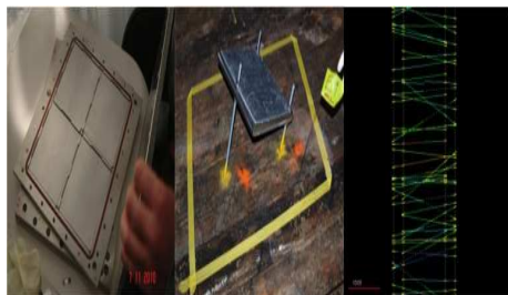
Figure 8: Left: emulsion module hosting 16 emulsions. Middle: module station during data taking. Right: reconstructed passing-through tracks.
