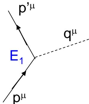
$$\begin{aligned} p^\mu &= p'^\mu + q^\mu \\ q^2 &= (p^\mu - p'^\mu)^2 = 2M^2 - 2p^\mu p'^\mu \\ &= 2M^2 \left( 1 - \frac{1 - \vec{v} \cdot \vec{v}'}{\sqrt{(1-v^2)(1-v'^2)}} \right) \\ &\leq 0 \text{ but } q^2 = m^2 ? \end{aligned}$$
