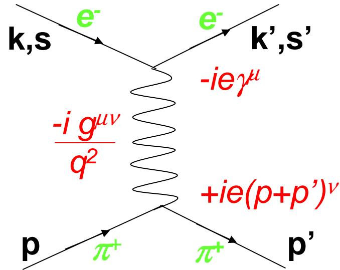
$$\begin{aligned} T &= \bar{u}(k', s')(-ie\gamma^\mu)u(k, s)\frac{-ig_{\mu\nu}}{q^2}(+ie)(p + p')^\nu \\ &= \frac{-ie^2}{q^2}\bar{u}(k', s')\gamma^\mu u(k, s)(p + p')_\mu \end{aligned}$$
