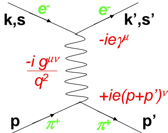
$$d\sigma = \frac{1}{2E_k 2E_p |\vec{v}_k - \vec{v}_p|} \int (2\pi)^4 \delta^4(k' + p' - k - p) \overline{|T_{fi}|^2} \frac{d^3 k'}{(2\pi)^3 2E_{k'}} \frac{d^3 p'}{(2\pi)^3 2E_{p'}}$$
